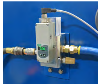
AFPCS Pump Control Mounted to Filter Press
