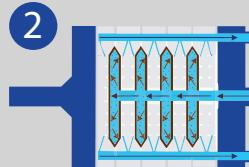
Solids begin to build on the filter cloth, trapping the ensuing particles and building a filter cake. The filter cake acts as a depth filter for solid/liquid separation. Filtrate exits the plates through the corner ports into the manifold.
