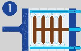
Slurry is pumped into the filter press. The solids are distributed evenly on the filter cloths during the feed (fill) cycle.
