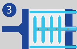
When the correct valves in the manifold are open, the filtrate exits through the filtrate outlet. As the feed pump builds pressure, the solids build within the chambers until they are completely full of filter cake.
