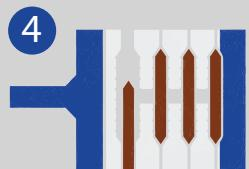
Once the chambers are full, the fill cycle is complete and the filter press is ready to be emptied.
