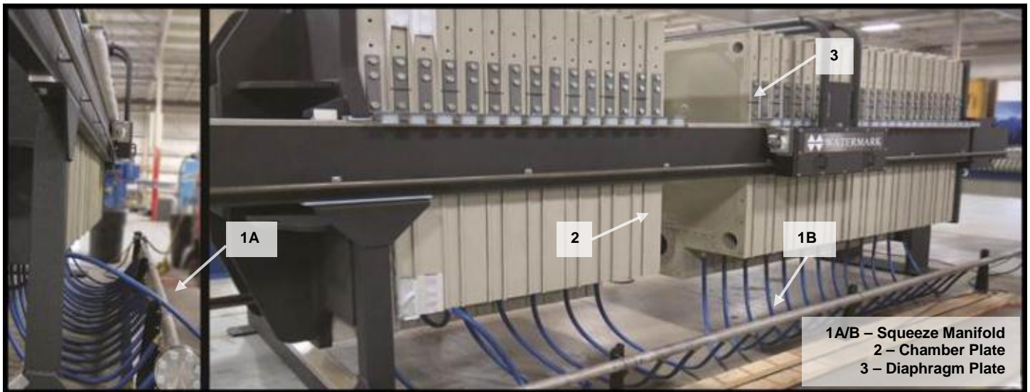
Diaphragm squeeze press with "mixed pack" plate stack.
