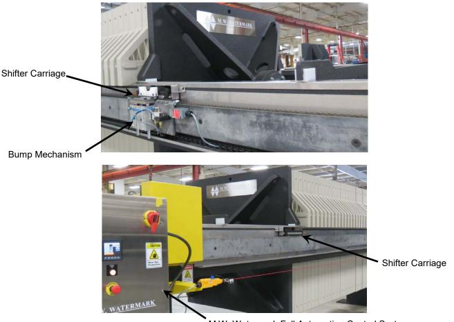
View Automatic Shifter & Automatic Shifter with "Bump" in Operation
