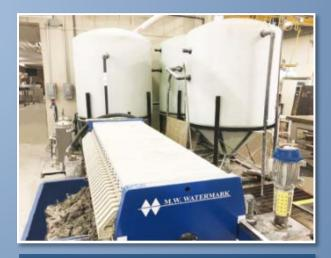
Capital Granite is using an M.W. Watermark filter press to help recycle the process/ waste water that is used throughout their fabrication shop.
