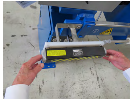
The Safety Buttons on Each Side Are Recessed to Help Prevent Operator Override
