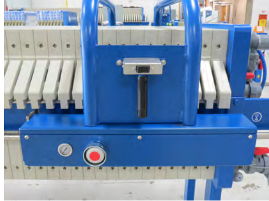
M.W. Watermark 630mm Filter Press with Optional Two-Hand Shifter Safety Interlock
