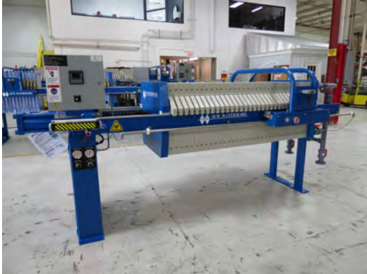
M.W. Watermark 630mm Filter Press with Optional Two-Hand Shifter Safety Interlock
