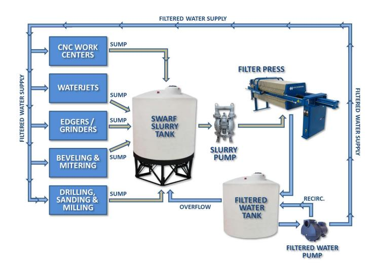
M.W. WATERMARK - Equipment and Service for Filtration, Process, and Dewatering Needs
