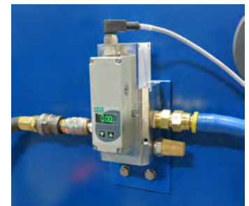
AFPCS Pump Control Mounted to Filter Press
