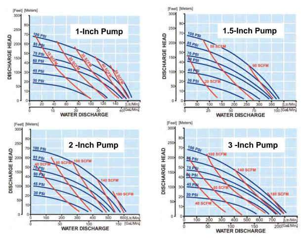
Standard materials of construction are either cast iron or polypropylene with Santoprene diaphragms. All curves are based on 1-ft flooded suction, Fluid viscosity 1 cps.
