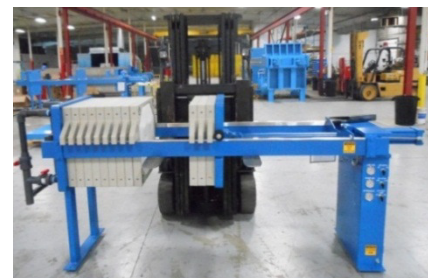
Figure 2: Lifting Press with Fork Lift
