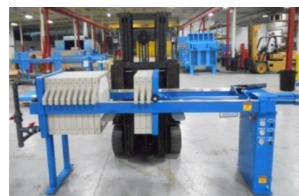
Figure 1: Press Rigging Using Sidebars 800mm and Smaller Presses
