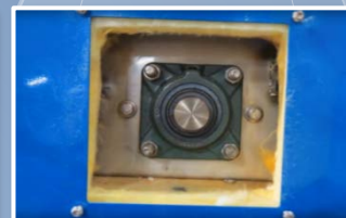
Easy External Access to High-Temperature Bearings
