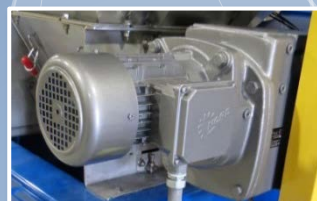
Oversized Extruder Gearbox with AC Drive and Inverter Duty Motor
