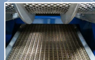
Stainless Steel Construction of All Wetted Components
