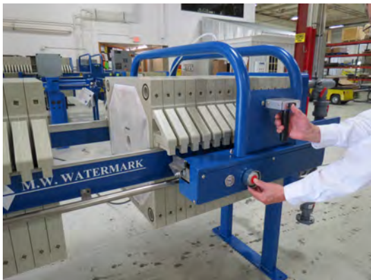
The Optional Shifter Safety Interlock Requires Both Hands to Be Used to Shift the Filter Plates A Guard Around the Safety Button Helps Prevent Inadvertent Activation
